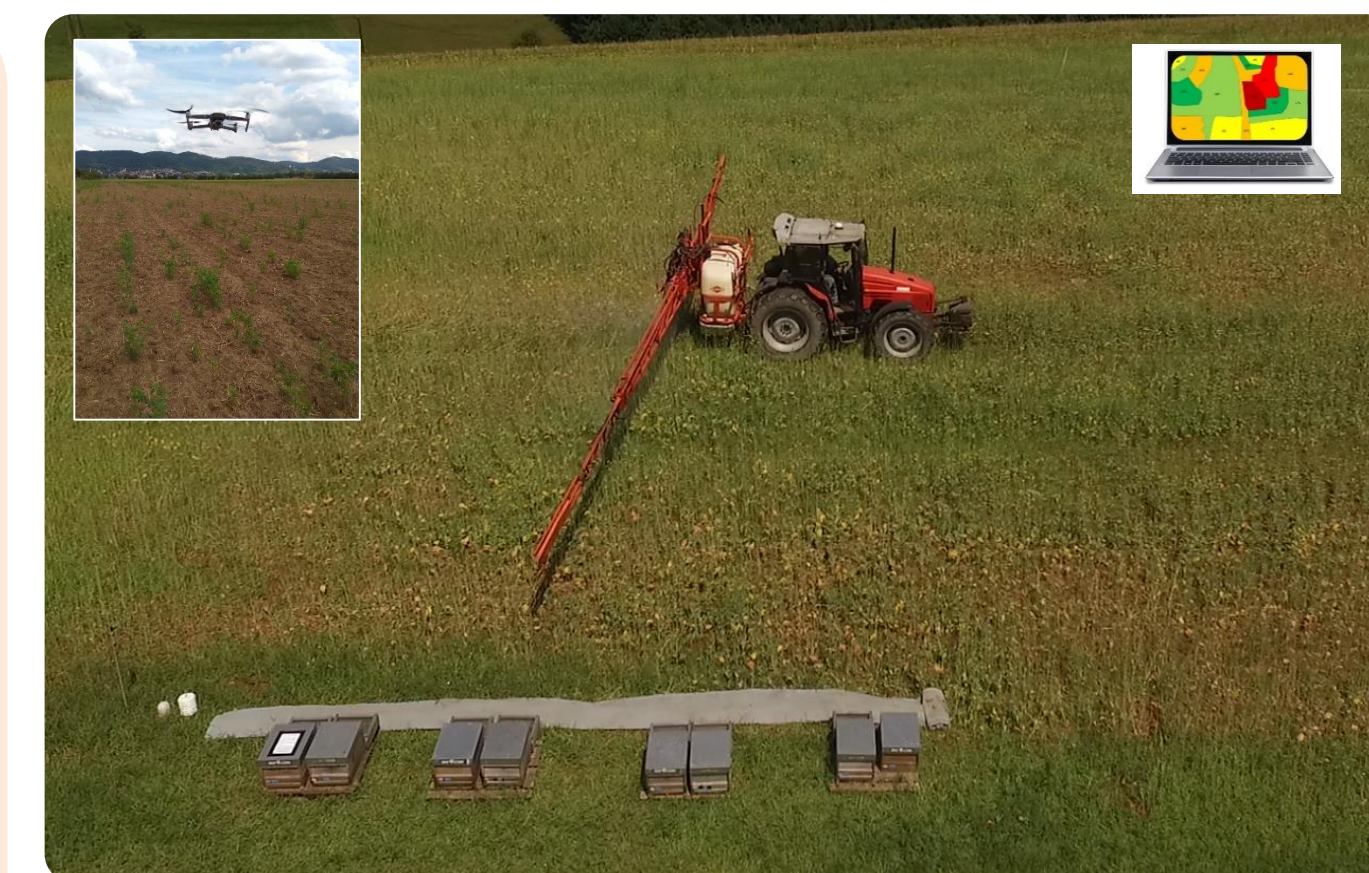
Figure 1: Example of precision application; weed-mapping via drones, data analysis followed by infestation orientated patchy herbicide application
